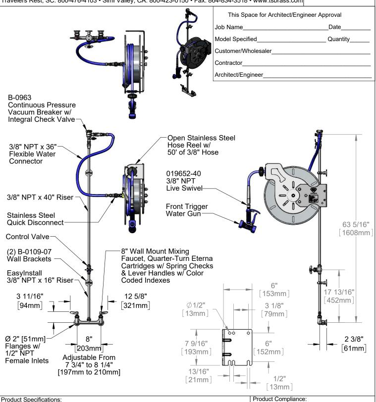
Open Stainless Steel Hose Reel w/ 50' of 3/8" Hose, Blue Front Trigger Water Gun w/ Swivel, Vacuum Breaker, 3/8" NPT Flexible Water Connector, 8" Wall Mount Mixing Faucet & Control Valve
