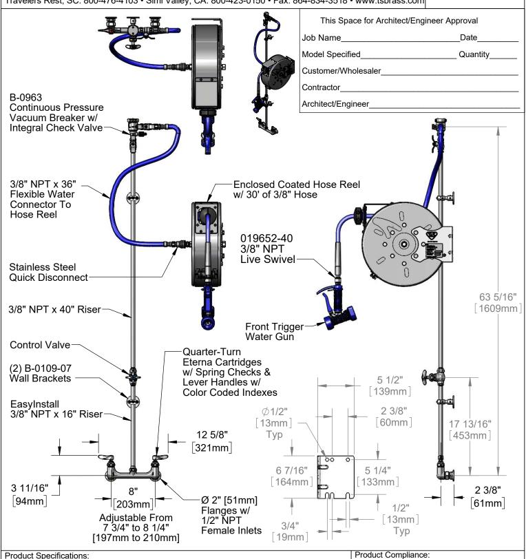
Enclosed Coated Hose Reel w/ 30' of 3/8" Hose, Stainless Steel Front Trigger Water Gun w/ Swivel, Vacuum Breaker, 3/8" NPT Flexible Water Connector, 8" Wall Mount Mixing Faucet & Control Valve
