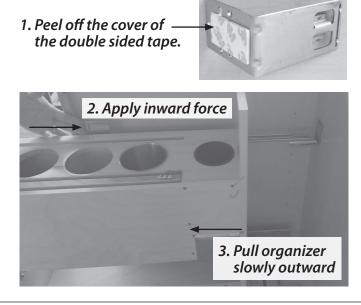
First, peel off the cover of the double sided tape at the back of the rear L-Bracket. Then applying an inward force at the front L-Bracket to ensure the rear L-Bracket has a firm contact with the cabinet back panel. While holding at the front L-Bracket, slowly pull the organizer halfway to gain access to the release clip to release the organizer from the slide base.
