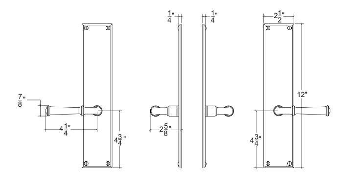
**Mortise Lock** standard backsets are 2-1/2" and 2-3/4" **Tubular Latch** standard backsets are 2-3/8" and 2-3/4" Can work with 2-1/8" face bores
