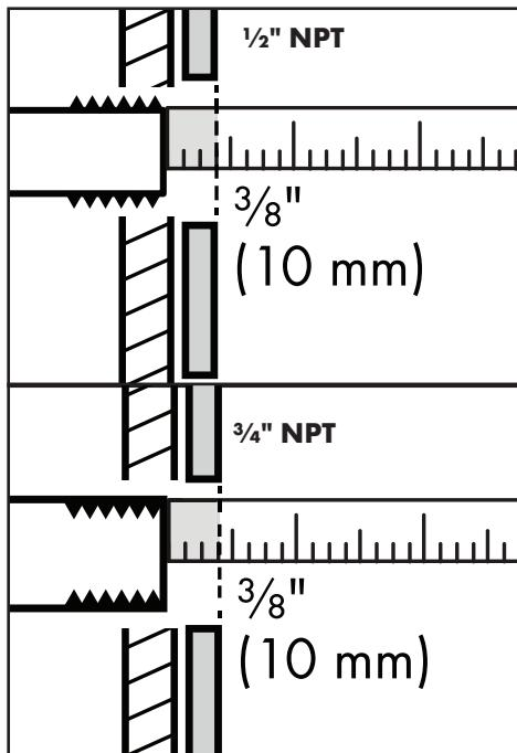
The tub spout requires either a 3/4" NPT female fitting or a 1/2" NPT male nipple recessed 3/8" (10 mm) behind the surface of the finished wall.
