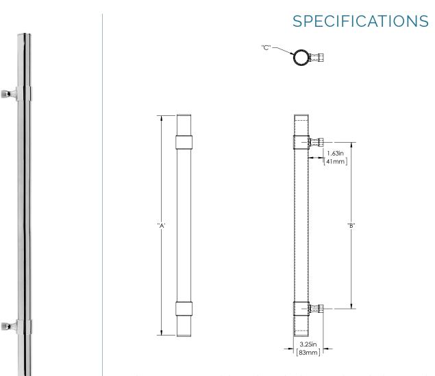
**Product Description:** 1 1/2" Tubular Round Grip with End Caps in Stainless Steel and Wrap Around Hourglass Mounts in Brass
