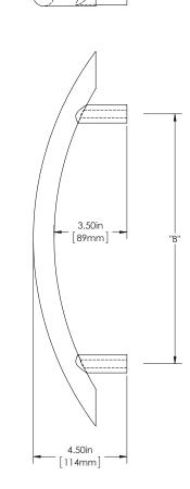
**Product Description:** 1" Tubular Round Front Curved Grip with Mitered and Welded Ends and Straight Round Mounts in Brass
