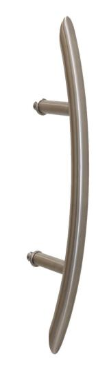
**Product Description:** 1" Tubular Round Front Curved Grip with Mitered and Welded Ends and Straight Round Mounts in Stainless Steel
