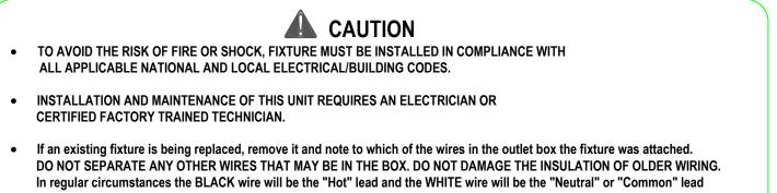
A GREEN or BARE COPPER wire is the "Ground". In older buildings it is always good practice to reconfirm the polarity of the wiring.
