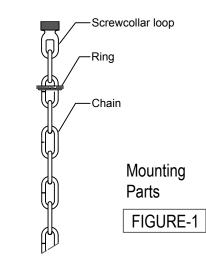
3. Open the end links of the chain. Attach the chain to the screw collar loop. Hang the fixture on the chain at the desired height. Remove excess chain. Close the chain links. Unscrew the ring from - the screw collar loop. Allow the ring and canopy to slide down the chain to the fixture.
