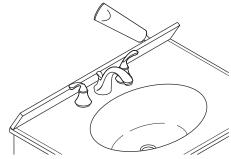
FINISH BY APPLYING A BEAD OF CAULK ALONG THE SEAM OF THE WALL AND THE VANITY TOP.
