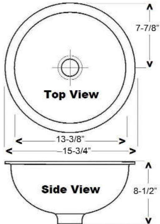
Dimensions of fixture are nominal and may vary within the range of tolerances established by ASME Standard A112.19.2. Dimensions and specifications subject to change without notice.
