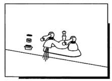
6. After installing faucet, remove aerator assembly and open the hot and cold water supplies. Check for leaks. Turn on faucet handle for one minute to flush debris from faucet. Close the handles and re-assemble the aerator.
